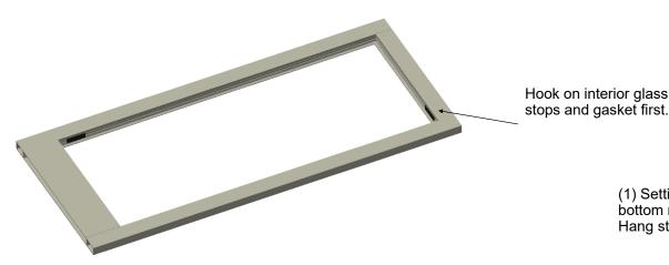
Back off glass jacks before installing glass. Tighten after glass is in place.
