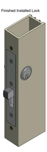
Attach face plate, cylinders, retaining pins, and any lock components per lock manufacture's instructions.
